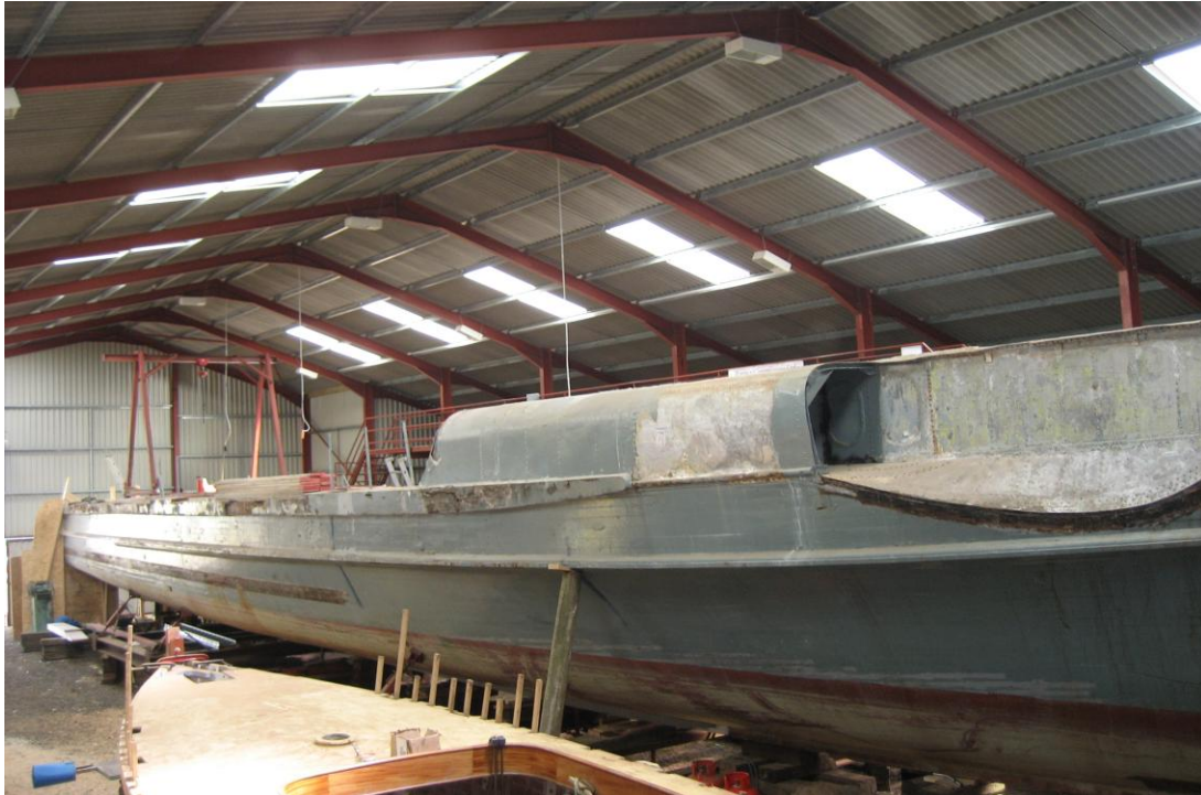
S130 looking from the bow to the stern, note the exit from this torpedo tube now the blanking plate has been removed and the sleek lines of the hull.
